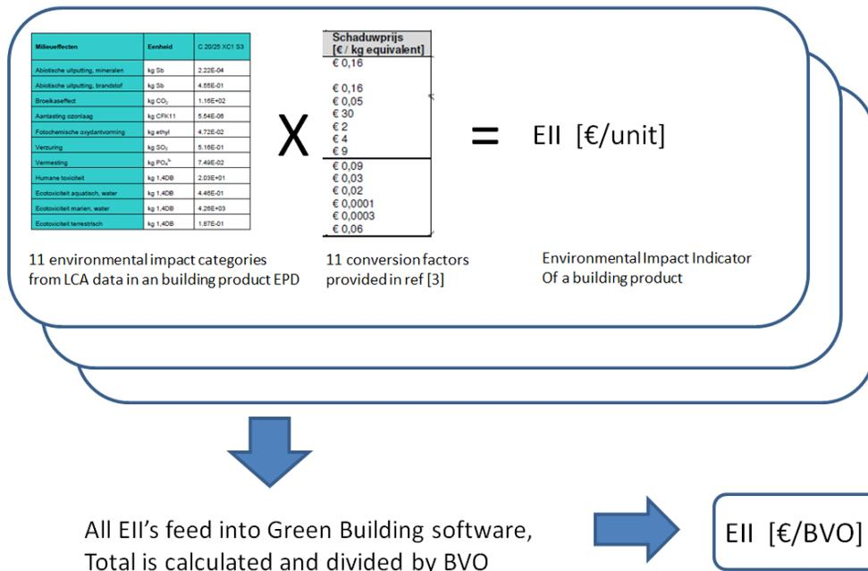
**Figure 2:** Schematic flow diagram to get from LCA data in a product EPD to the EII of a building product and from there to the EII of a construction work
