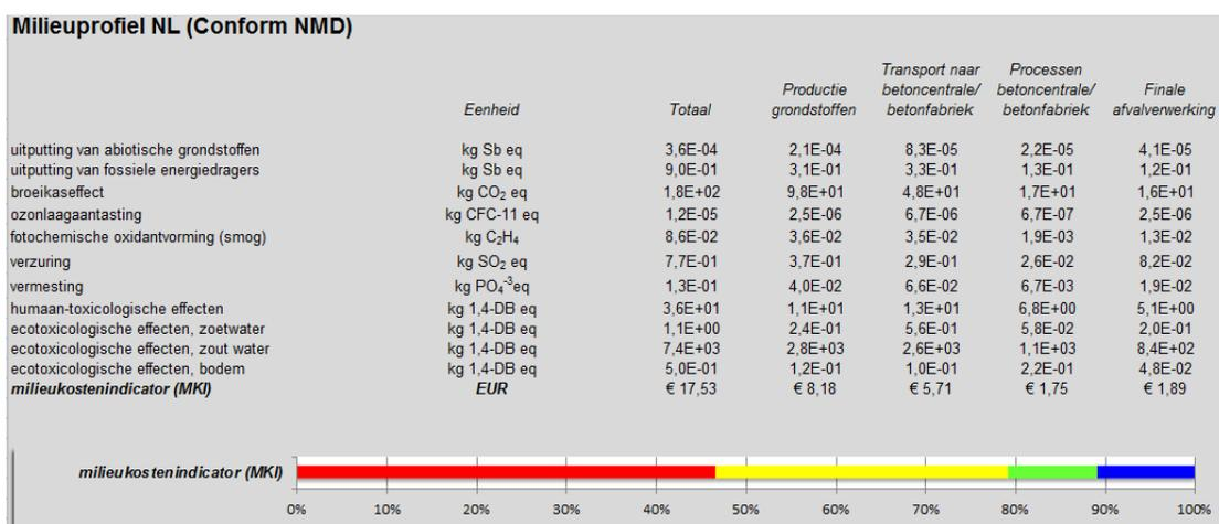
**Figure 4:** The EII (MKI in Dutch) built up by the environmental impact effects and by process phase (red: raw materials, yellow: transport raw materials to concrete plant, green: concrete plant process, blue: end of life scenario concrete)
