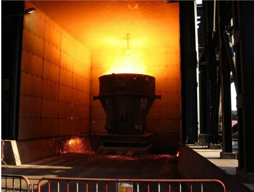
**Figure 3:** Stand for injection of sand+O<sub>2</sub>/N<sub>2</sub> in molten converter slag in AM Gent<sup>3</sup>
