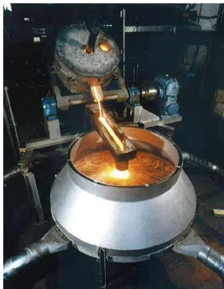
**Figure 7:** Pilot for the spinning disk technology by Siemens-VAI<sup>14</sup>
