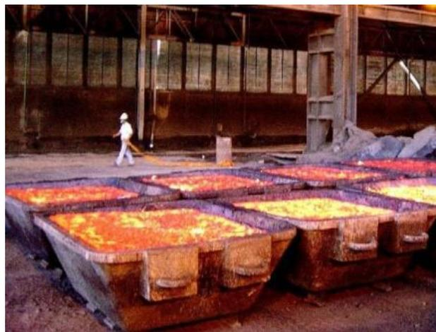
**Figure 6:** Steel moulds for BOF slag cooling in China Steel Corporation (Taiwan)
