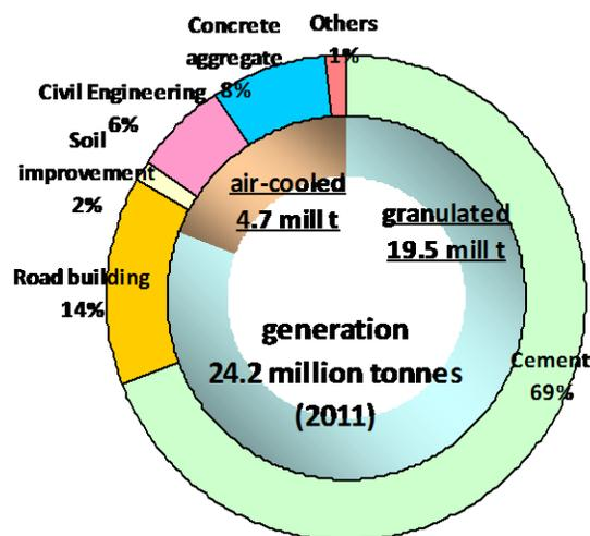
Figure 3: Breakdown of BF slag usage, total generation and the ratio of granulated and air-cooled (2011)<sup>1</sup>
