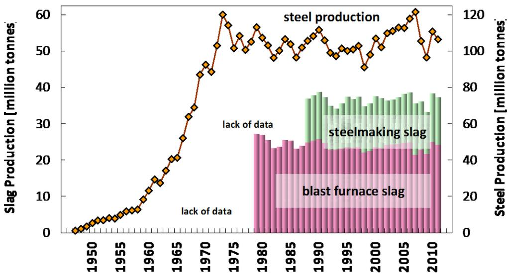
Figure 1: Annual production of slag<sup>1</sup> and steel<sup>4</sup> in Japan
