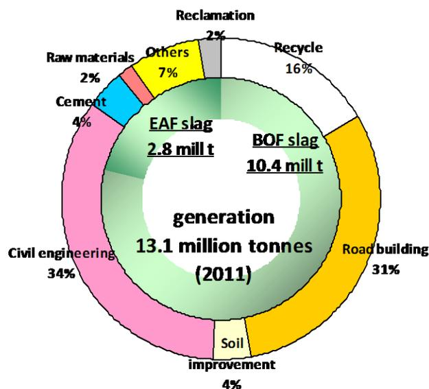
**Figure 4:** Breakdown of steelmaking slag usage, total generation and the ratio of BOF and EAF slag (2011)<sup>1</sup>
