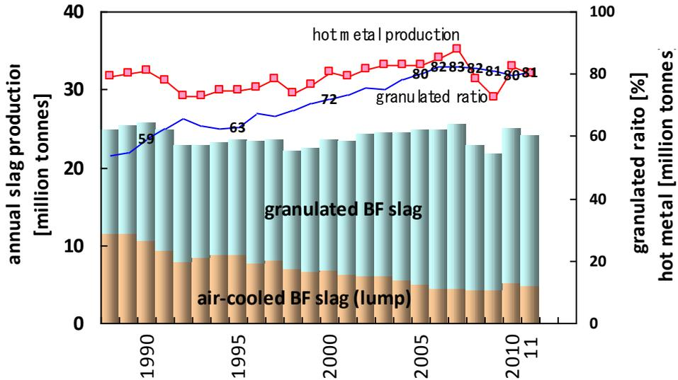
Figure 2: Change of granulation ratio of BF slag<sup>1</sup>
