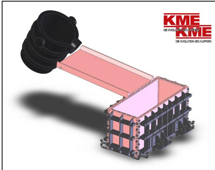
**Figure 5:** Scheme of slag solidification by DEWEOS technique
