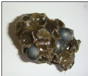
**Figure 1:** Fully vitrified blast furnace slag after cooling with Paul Wurth-system
