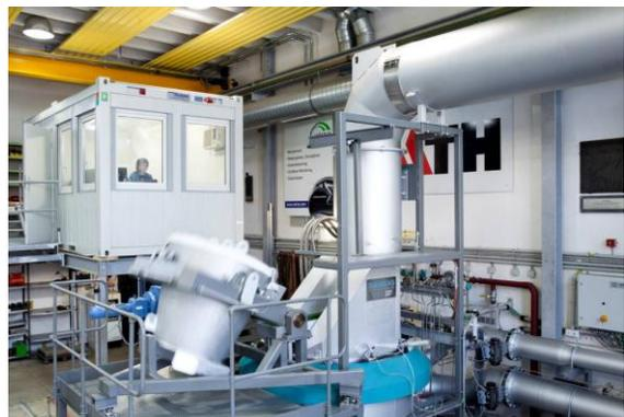
**Figure 3:** Technical plant of DSG-rotating cup at Montan University Leoben (MUL)
