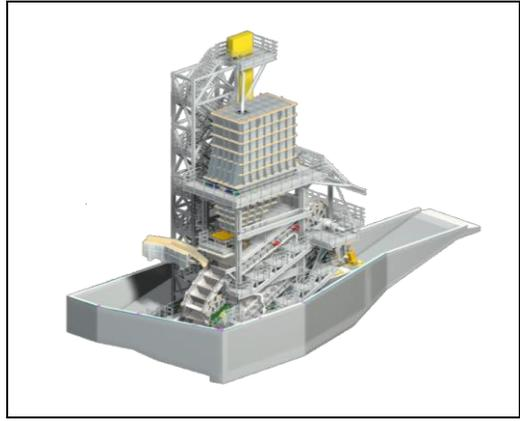
**Figure 2:** Large scale test series at Dillinger Hütte (ROGESA) and planned slag caster with steel sphere storage hopper for the upcoming pilot plant to be built at Dillinger Hütte BF No. 4 with a capacity of up to 6 t/min of liquid blast furnace slag
