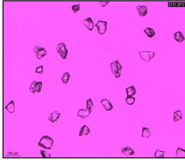
**Figure 4:** Fully vitrified blast furnace slag after cooling with Siemens-system
