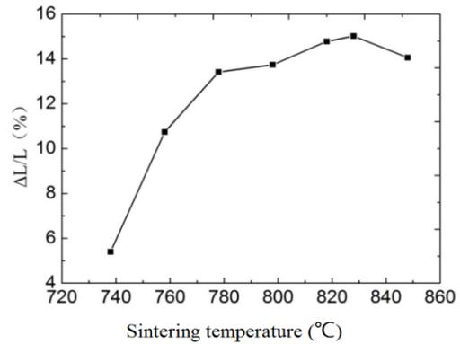
**Figure 2:** Sintering shrinkage rate with increasing temperature
