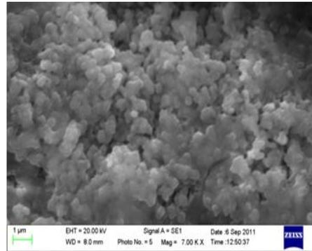
**Figure 4:** SEM photographs of glass ceramic
