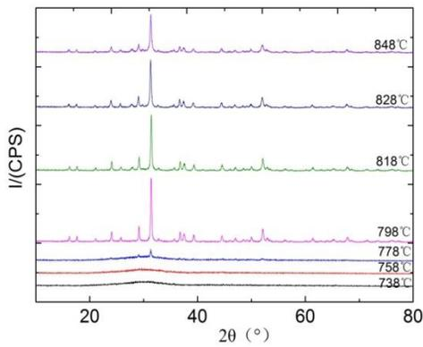
**Figure 1:** XRD patterns of the sintering samples at different temperature for 1h
