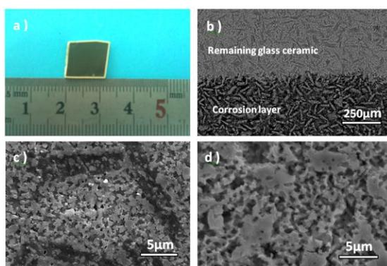
**Figure 1:** The macro and micro morphology pictures of the cross section surface of the sample after etched in HCl solution (pH=1) at 85°C for 5 days: a) Macro image of the cross section of the bar shaped sample; b) BSE photo of dilute HF etched cross section of the bar; c) SE image of the remaining glass ceramic and d) the corrosion layer
