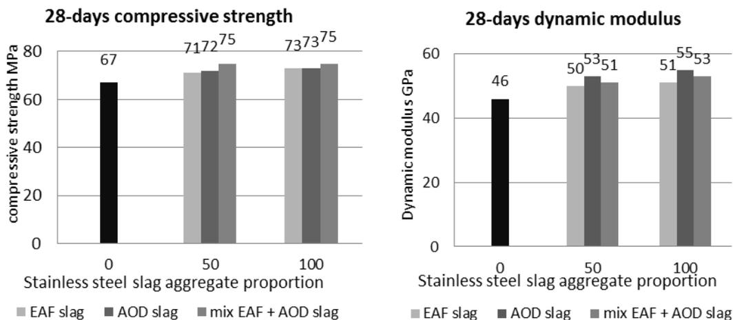
Figure 1: Compressive strength and dynamic of concretes
