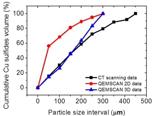
**Figure 3:** Cumulative copper sulfide volume versus copper bearing particle size plotted with CT scanning and QEMSCAN data before and after 3D transformation<sup>4</sup>
