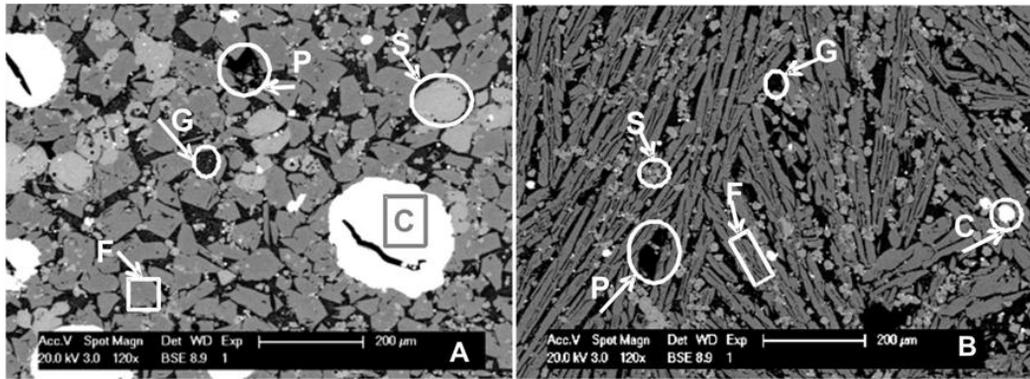
**Figure 1:** SEM-Backscattered Electron (BSE) image of copper slag: (F) fayalite; (S) magnetite (spinel); (G) glass; (C) copper sulfides; (P) pores<sup>3</sup>
