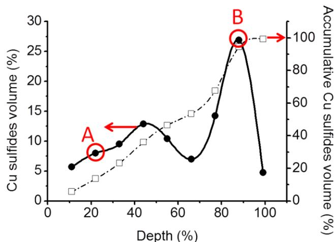
**Figure 2:** Copper sulfides volume distribution along depth of slag layer: (A) section near the top of slag layer; (B) section near bottom of the slag layer<sup>4</sup>
