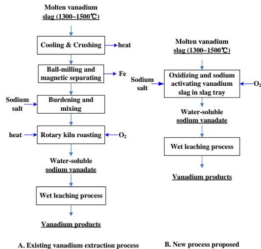
**Figure 1:** Flowchart of the existing vanadium extraction process and the new process
