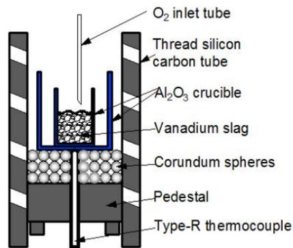
**Figure 2:** Experimental apparatus profile
