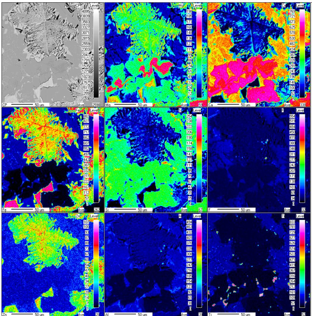
**Figure 2:** Elemental mapping of the 25 wt% fayalite (with CaF<sub>2</sub>) modified AOD slag
