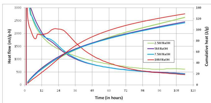
Fig 1 Calorimetry of CtCS\_45\* with NaOH at 80°C
