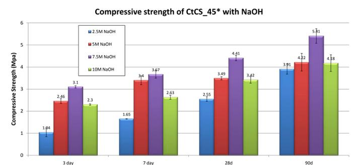
Fig 2 Compressive strength of slag mortars with different NaOH solutions
