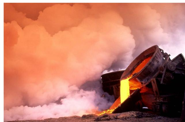
Tapping of a steel slag pot at the slag yard. At this moment, most of the slag's properties have already been determined by choices made during the high-temperature process.
