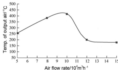
**Figure 7:** The average temperature of output air as a function of the air flow rate
