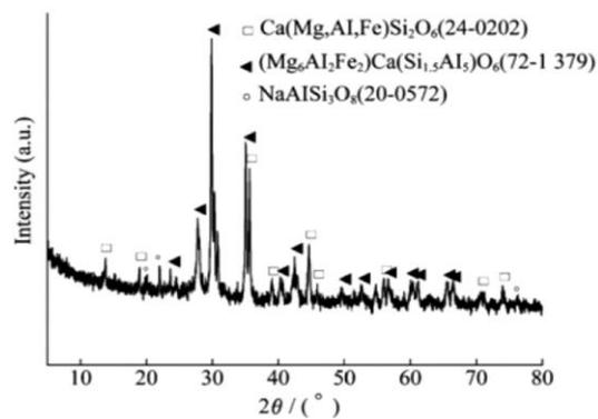
Figure 4: XRD patterns of glass-ceramics
