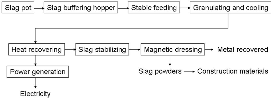
**Figure 1:** Schematic diagram of the slag treatment and energy recovery flowsheet for steelmaking slag
