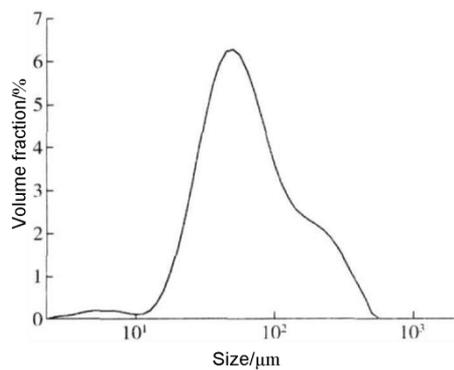
**Figure 2:** Particle size distribution of jetted steel slag
