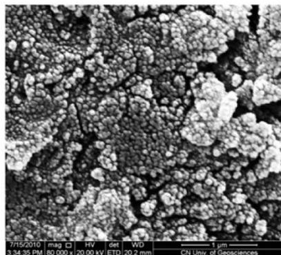
Figure 5: SEM image of glass-ceramics
