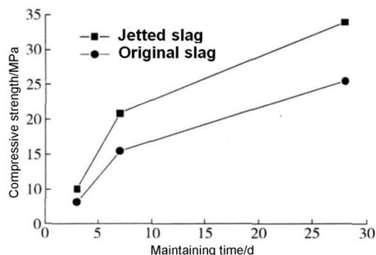
**Figure 3:** Comparison of compressive strength of cement samples from jetted and original steel slag
