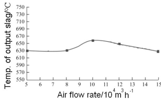
**Figure 6:** The average temperature of output slag as a function of the air flow rate
