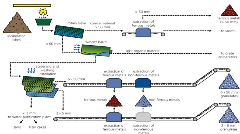
**Figure 3:** Schematic presentation of the wet separation process.
