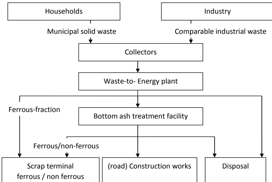
**Figure 1:** Flow chart, explaining the mass flow from origin to final destination<sup>1</sup>
