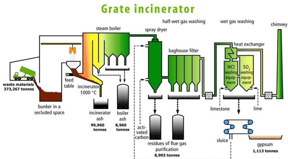
**Figure 2:** Schematic representation of the MSWI Waste-to-Energy plant in Doel
