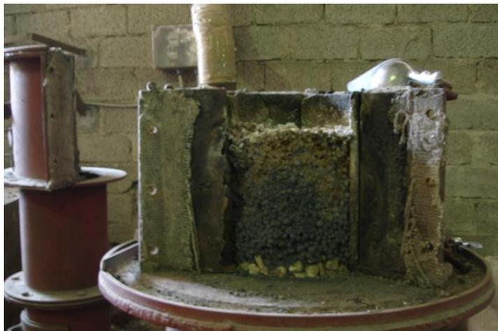
**Figure 1:** Sinter pot open after firing; the porous cake appears in the center
